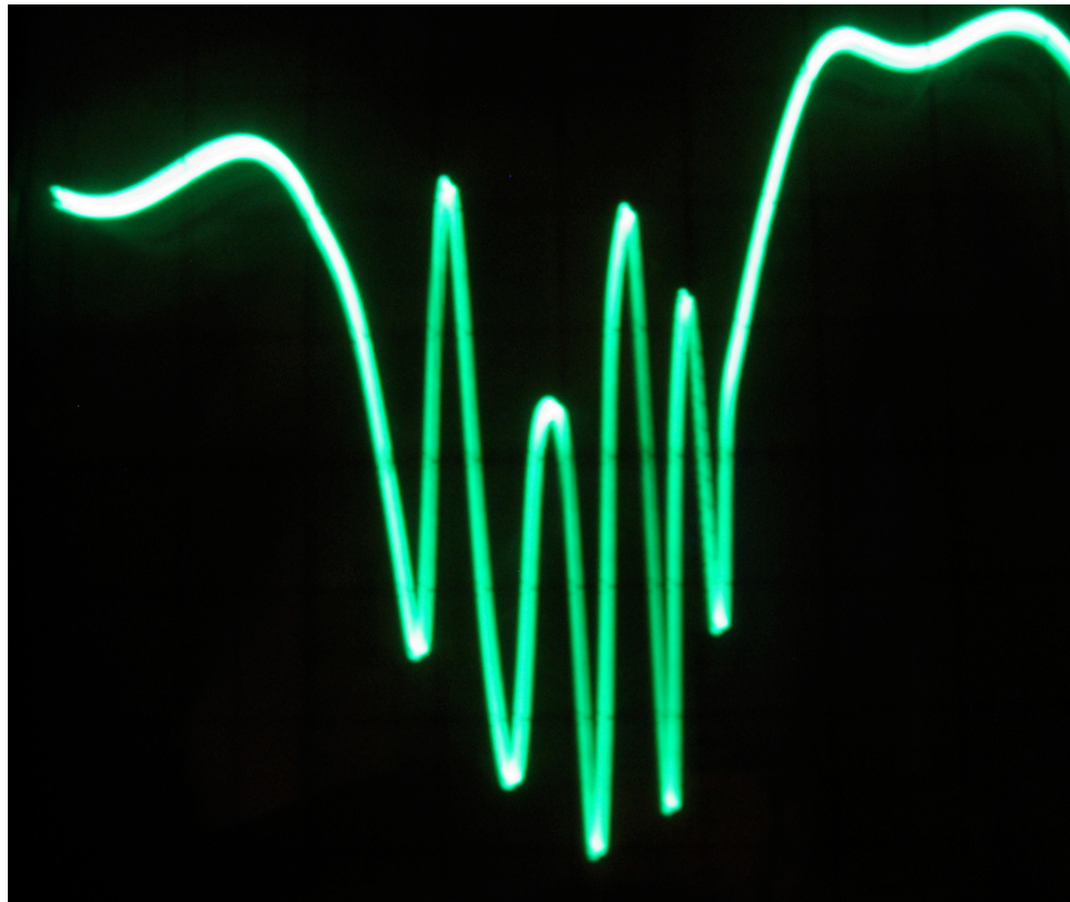
Figure 4.3: Doppler-Free DAVLL signal. The reference laser is tuned across the F_g = 3 \rightarrow E transitions. F_g = 3 \rightarrow F_e = 2 is the right-most transition, and F_g = 3 \rightarrow F_e = 4 the left-most. In between we see F_g = 3 \rightarrow F_e = 3 , and cross-over resonances.
